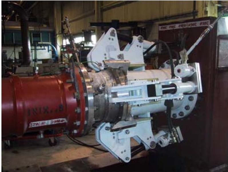
Figure 2.4.6.2-3 Quick Connect/Disconnect Coupling
