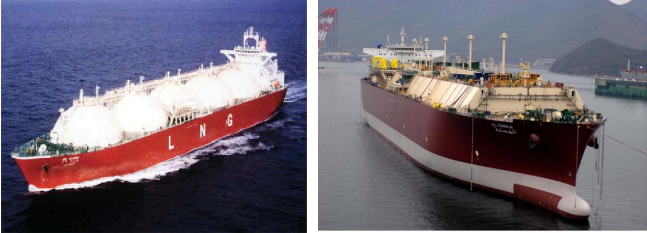
Kvaerner-Moss spherical tanks (left) (*Intertanko/Qatargas*) and membrane tanks in an LNG carriers (*Qatargas*)
